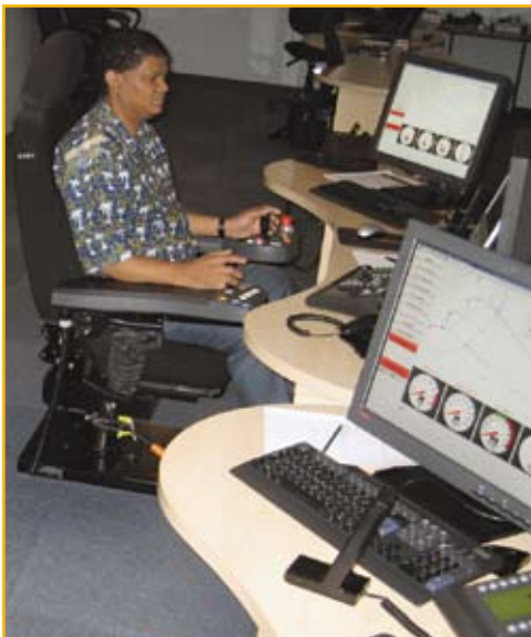
Remote loading of underground mining vehicles from surface control room.
