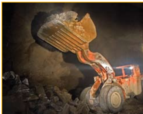
Loading out Cu-Ag-Pb-Zn ore from the Cozamin mine.
