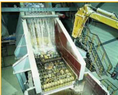
Pre-screening at the Wülfrath-Flandersbach plant.
