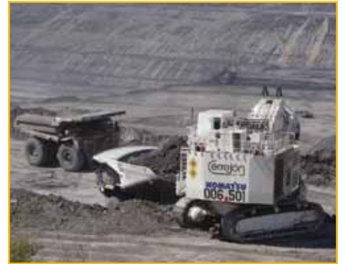
Waste rock excavation using hydraulic excavator and haul truck.
