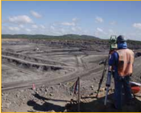
Surveying crew in one of the pits collecting data to update the mine’s grids.
