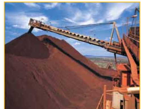
Stacking iron ore on to blending stockpile at Rio Tinto's Yandicoogina mine, Western Australia.
