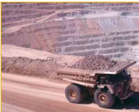
Haul truck transporting ore from Bingham Canyon mine to the Copperton concentrator.
