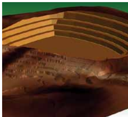
A pit design showing a push back into an existing topography with a draped texture.
